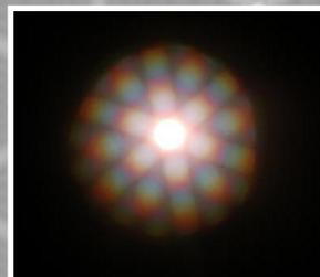
Fig. 4: Observation of the Sun with the ELSA configuration (main baseline of 24  $\mu\text{m}$  and hole diameter of 7.2  $\mu\text{m}$ ).
