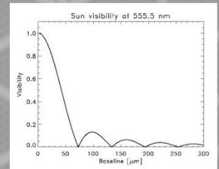
Fig. 1: Absolute visibility of the Sun with respect to the baseline length at 555.5 nm. The Sun is resolved for a baseline of about 70  $\mu\text{m}$ .
